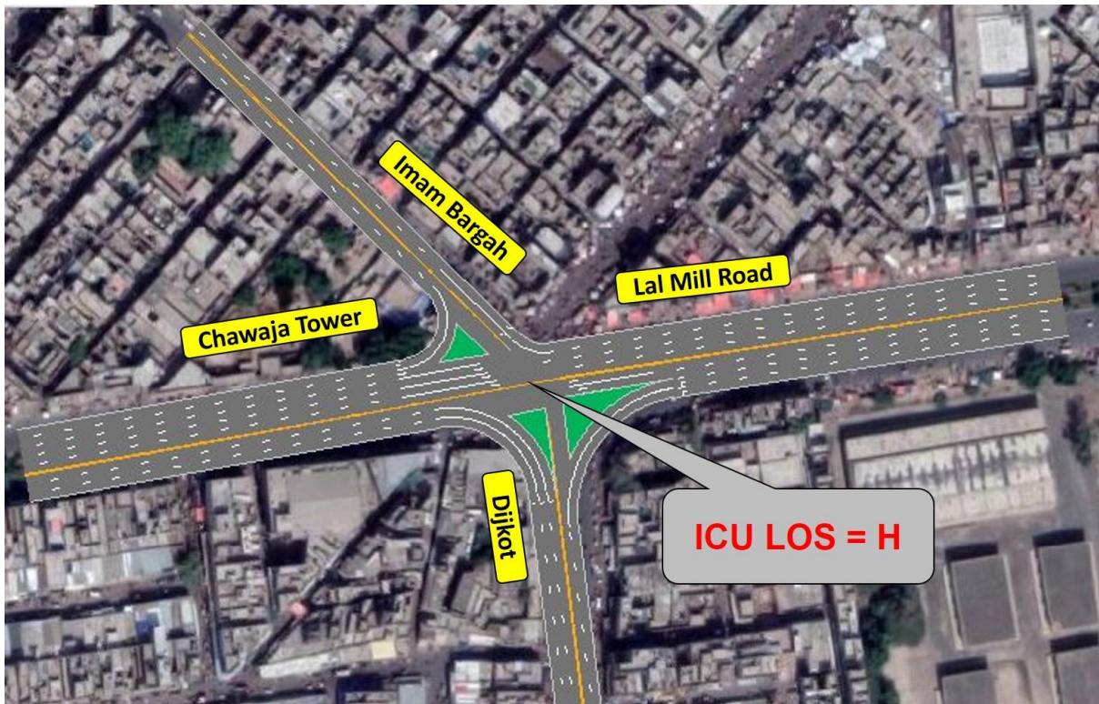
Figure 3-23: Existing Intersection of Minerva Cinema Chowk
